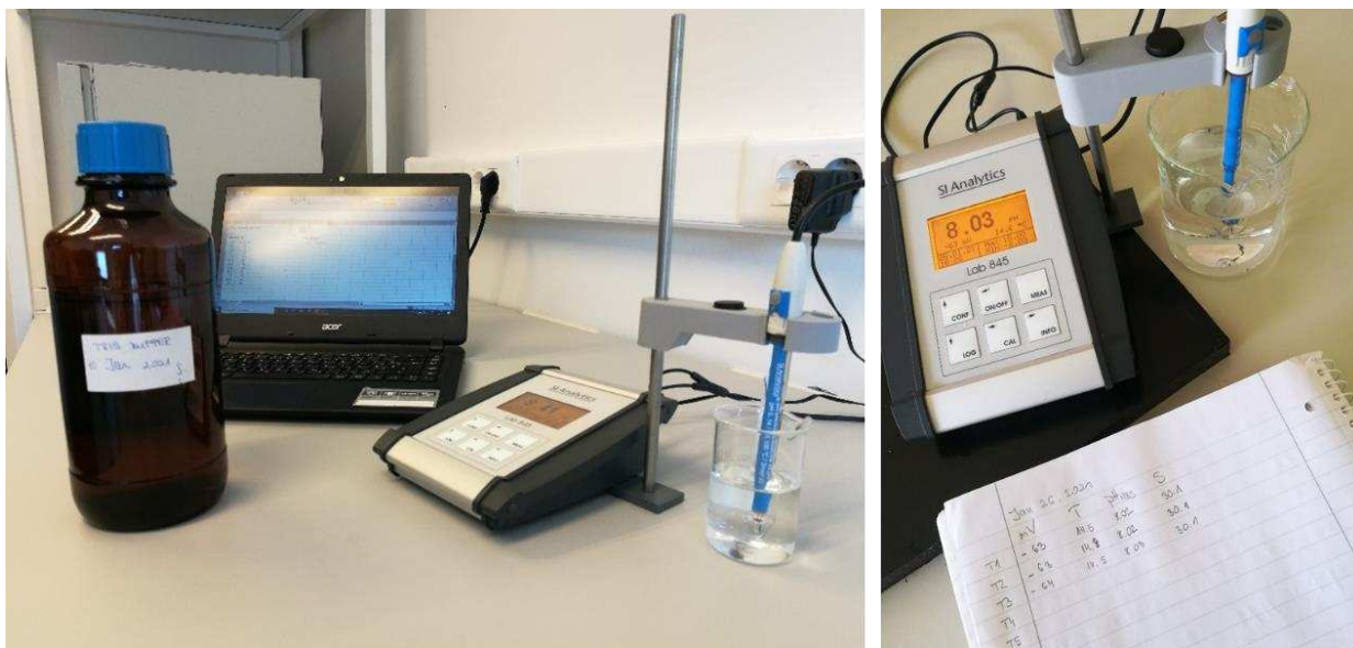
Figure 3.4.3.1 a) pH probe calibration with TRIS buffer), and b) experimental seawater sampling.
