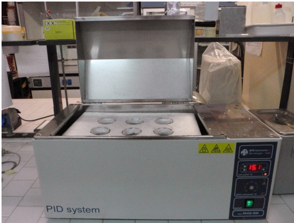
Figure 3.3.1.3 Programmable water bath with beakers placed inside.
