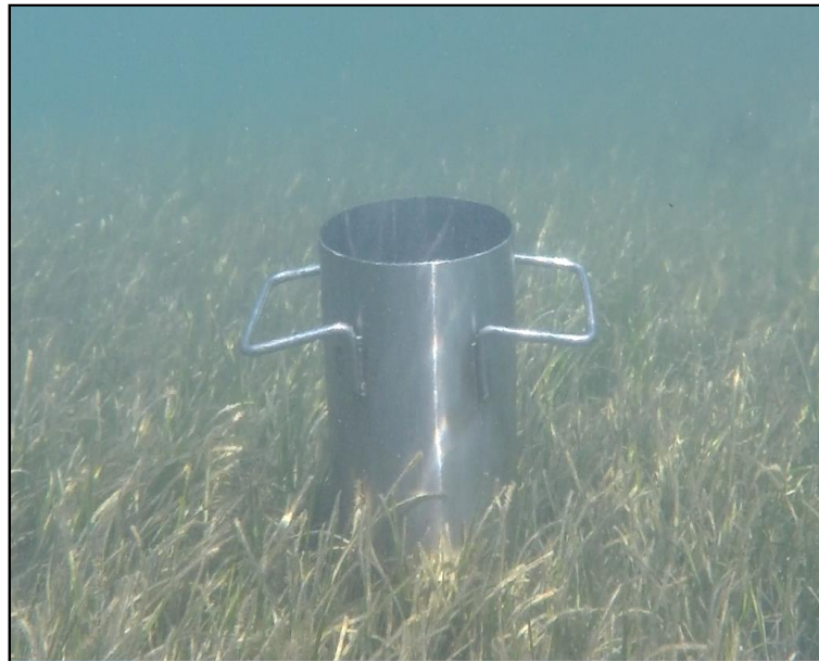
Figure 3.3.1. Seagrass corer used for seagrass sampling (photo: Melita Mokos).
