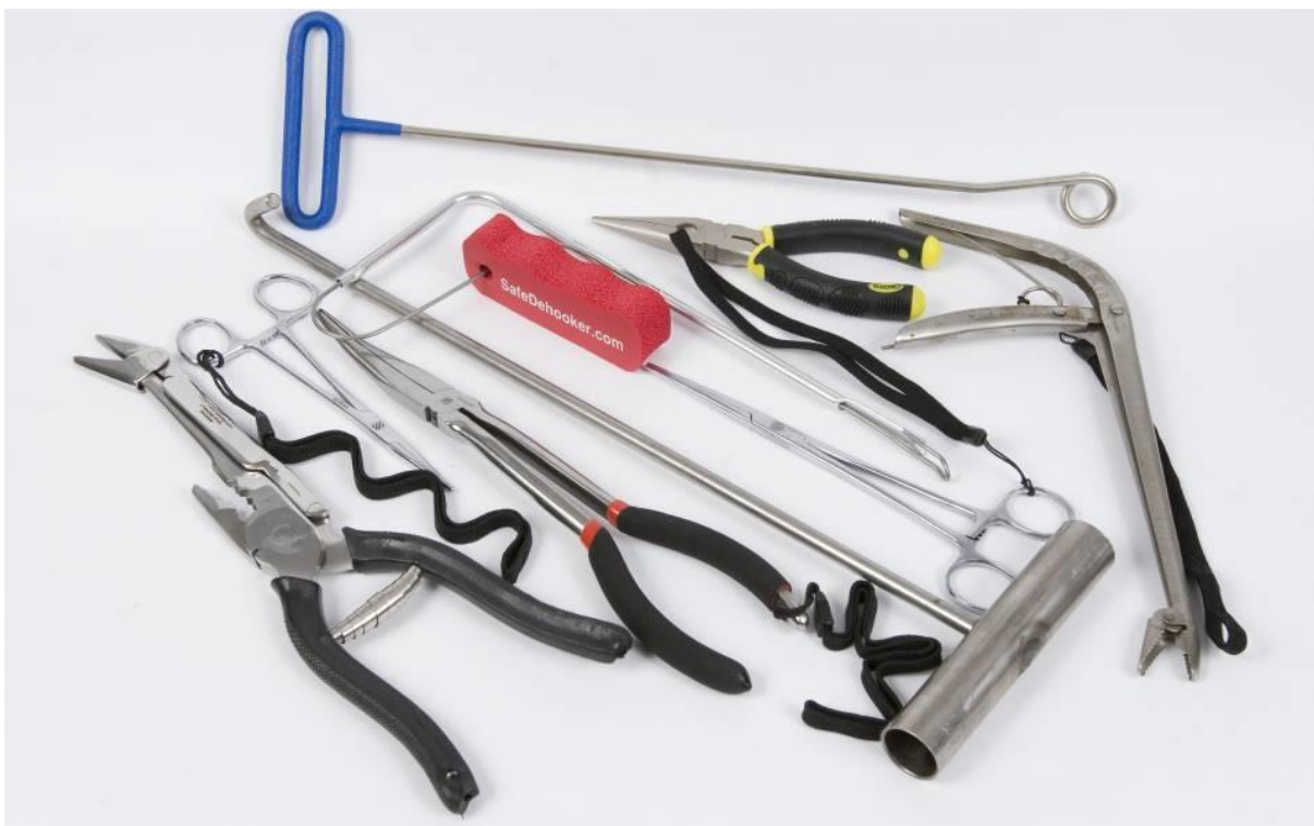
Slika 9. Različiti alati za vađenje udica (Izvor: http://4.bp.blogspot.com/-FRY1F0-7QbA/TVShXpBv9YI/AAAAAAAAA0M/j4wNXXN_hLE/s1600/variety+of+dehookers.jpg )
