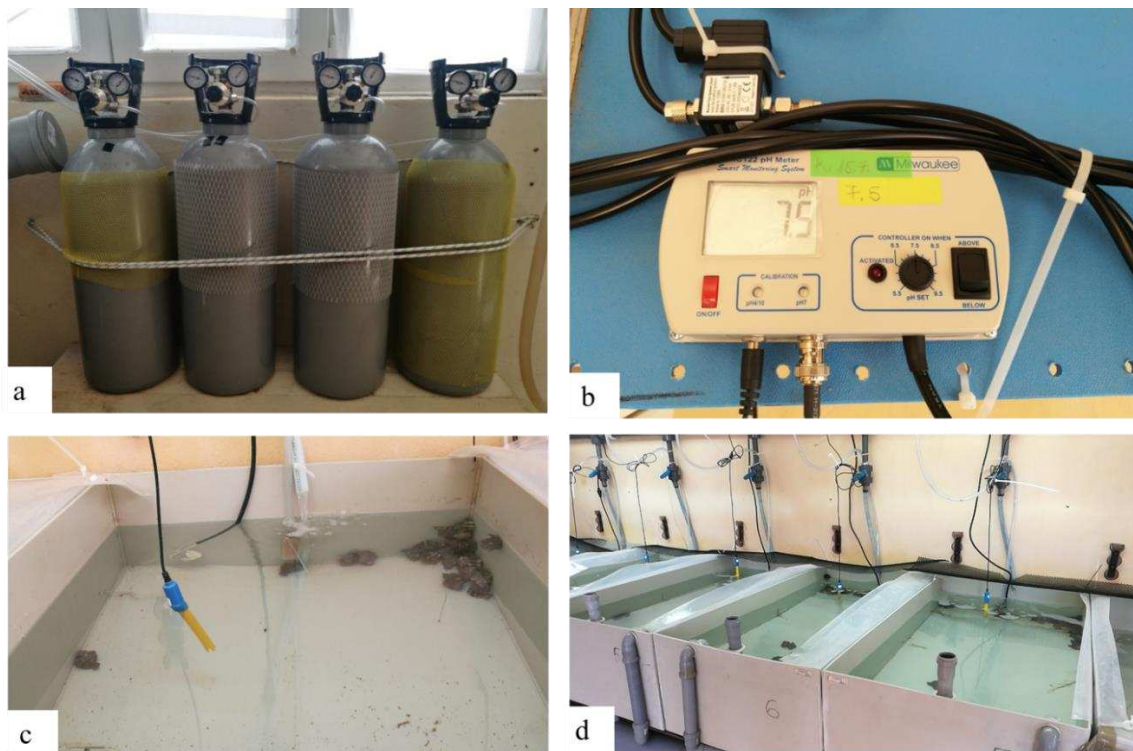
Figure 3.3.1 Equipment used in experimental system: a) CO 2 gas bottles; b) pH controller; c) pH probe; d) experimental tanks
