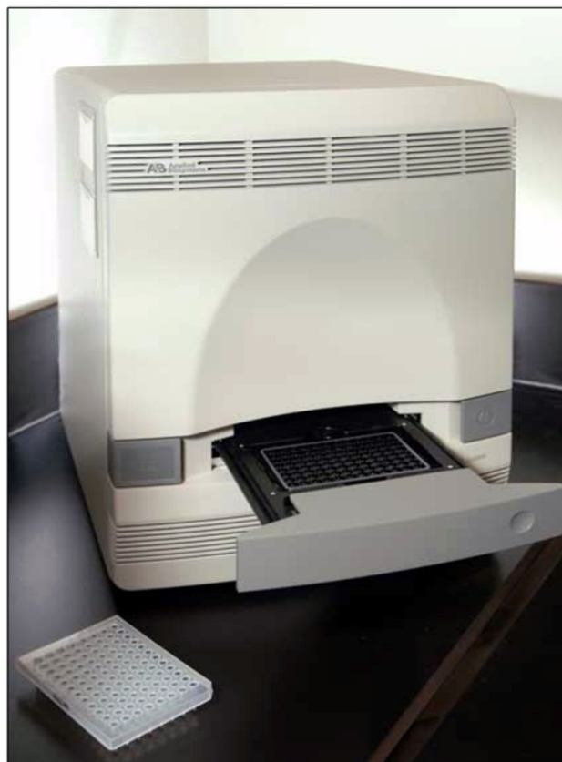
Figure 3.3.2.1 ABI 7500 Real-Time PCR System (Applied Biosystems, USA) used for PCR hsp70 gene expression analysis (source http://www.sequences.crchul.ulaval.ca/eng/appareils.html ).
