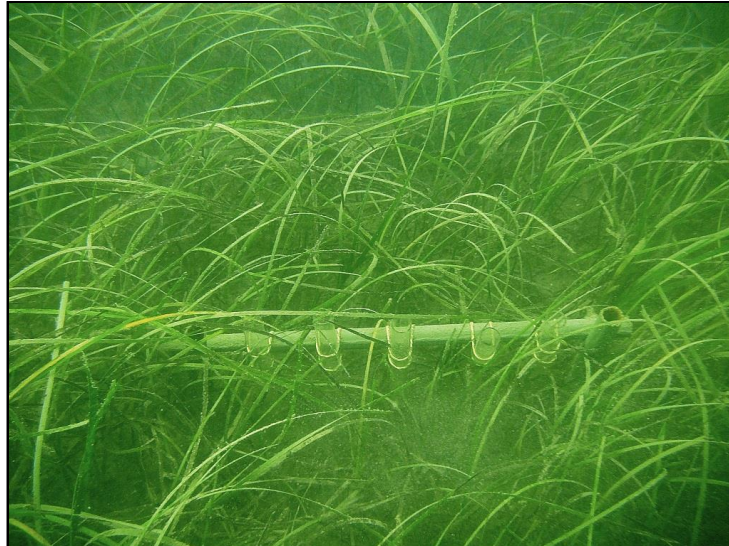
Figure 3.4.1. Sediment traps deployed on the sea bottom inside a seagrass meadow (photo: Melita Mokos).
