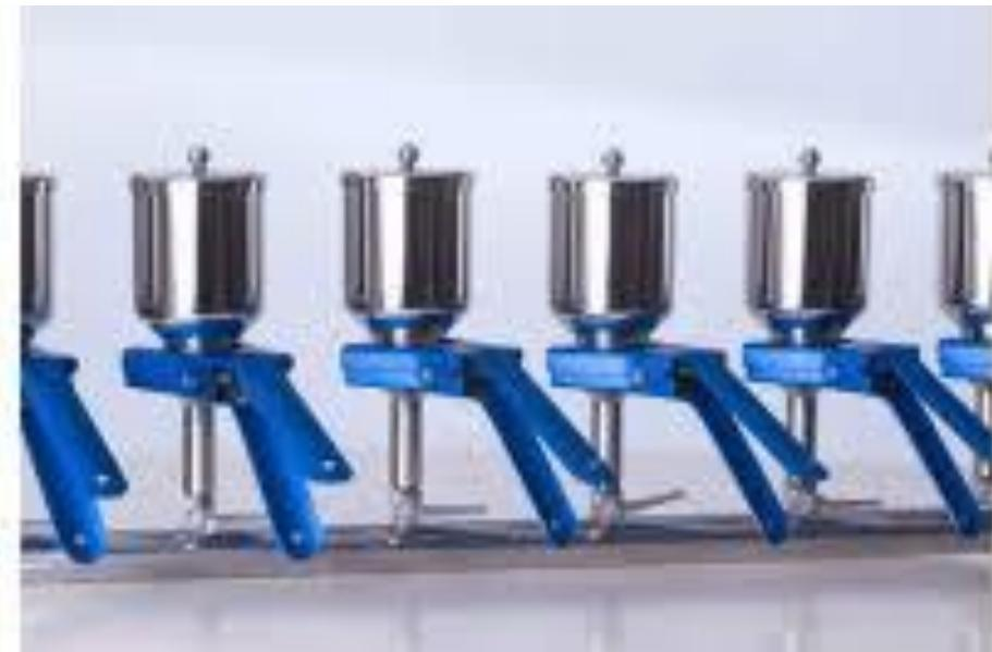
**Slika 9.** Aparatura membranske filtracije i držači filtera (plavo obojeni) (izvor: [http://tr.starlabsci.com/300ml-glass-3-branches-vacuum-filters\\_p77.html](http://tr.starlabsci.com/300ml-glass-3-branches-vacuum-filters_p77.html))
